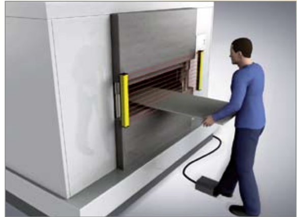
Floating blanking and fixed blanking as a standard function in the advanced model.
